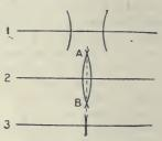
Instead of continuing to mark points until they finally reach diagram (iii), they will see that (ii) can be used immediately if the points A and B be joined; such appears to be the way in which the familiar method of bisecting a straight line arose. When a construction for bisecting an angle is required a little later, it can easily be invented by a slight modification of the above.
